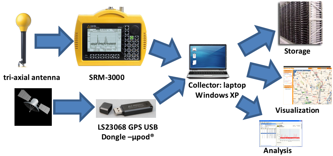
Fig. 6.2: Measurement Setup
