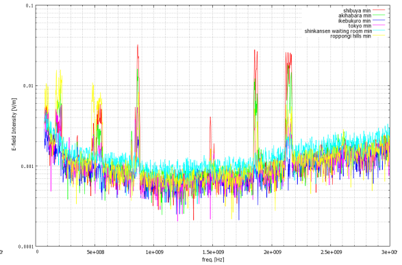
Fig. 8.44: Maximum RSSI of All Channels at All 6 Locations [75~3000][MHz]
