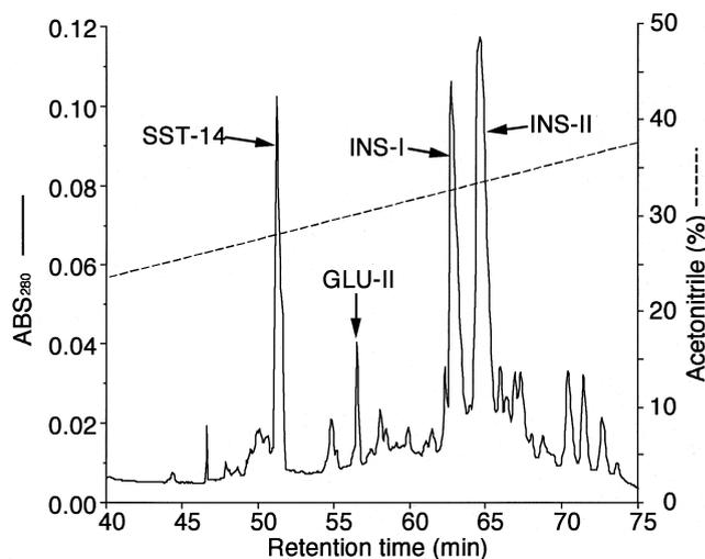
**Fig. 2.** Purification of pancreatic hormones fractionated by an ODS-120T analytical column. A µ RPC C2/C18 SC column was used. SST-14, GLU-II, INS-I and -II denote somatostatin-14, glucagon-II, insulin-I and -II, respectively.
