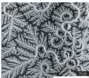
Figure 8.47: Split bent crystal of PCL in thin film [21].
