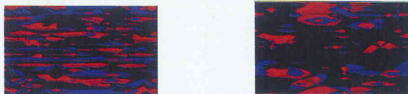
Fig 11 Contours of stream wise vortices at Re=180 , red=+50, blue=-50.
