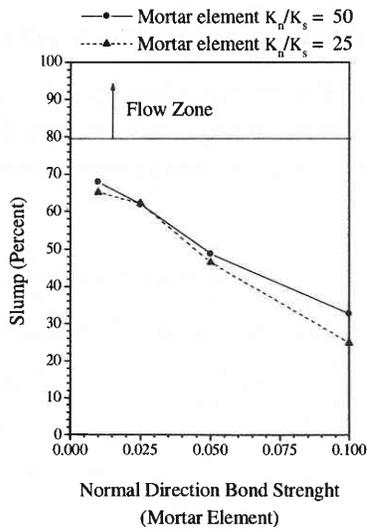
Fig. 7 Effect of bond on slump value.
