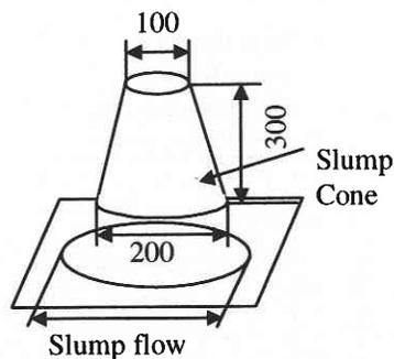
Fig. 1 Slump flow Test. Simulation sizes is half of this. (Dimensions in mm)
