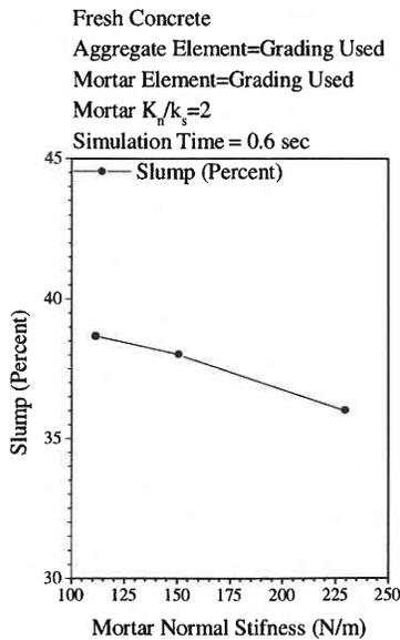
Fig. 4 Effect of mortar normal stiffness on slump value.
