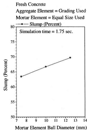
Fig. 5 Effect of mortar element ball diameter on slump value.
