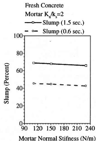
Fig. 3 Slump flow simulation.
