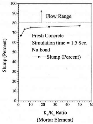
Fig. 6 Effect of stiffness ratio on the slump value.
