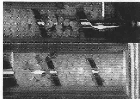
Fig. 4 Example of visualized image around the feed throat (168 rpm)
