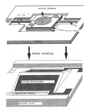
Fig.1 Functional diagram of a rotating antenna
