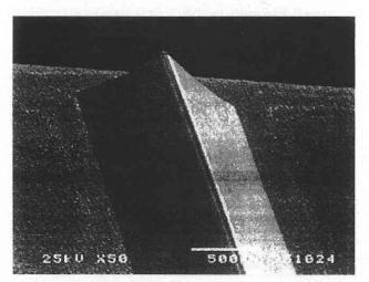
Fig.3 Triangular shape obtained by KOH etching
