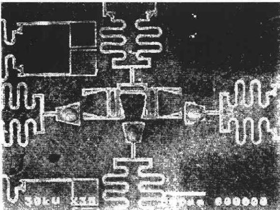
Fig.3 The XY stage
