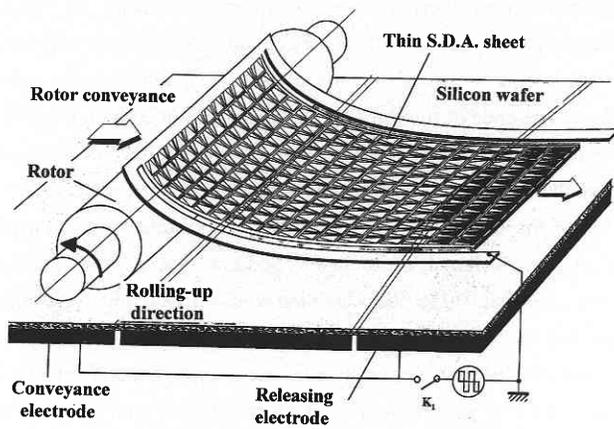
Fig.4 Hybrid fabrication principles of a macroscopic tubular motor.
