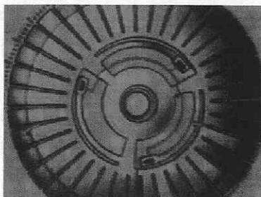
Fig.2 Annular electrostatic micromotor,  $\phi=500\mu\text{m}$ , 36 torsions beams and 3 buckling beams.
