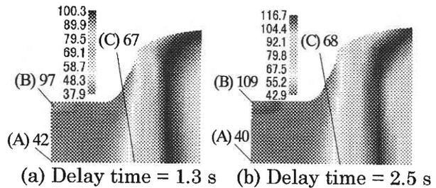
Fig. 6 Austenite grain size distribution at different delay times (a), (b)
