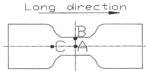
Fig. 2 Positions where grain size was measured
