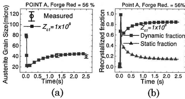
Fig. 4 (a) Transition of average grain size, and (b) Transition of recrystallized fraction at point A
