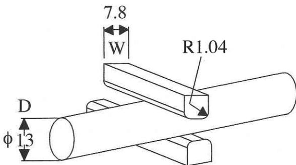
Fig. 1 Dimensions of the workpiece and plane dies
