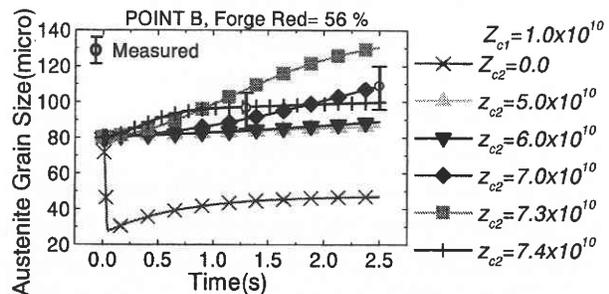
Fig. 3 Transition of average grain size at point B
