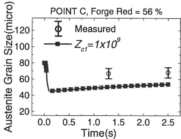
Fig. 5 Transition of average grain size at point C
