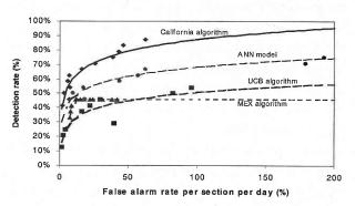
Fig. 1 Performance curves of the four incident detection algorithms
