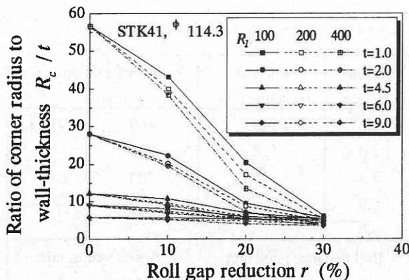
Fig. 4 Effects of  $r$ ,  $t$  and  $R_1$  on  $R_c$ .
