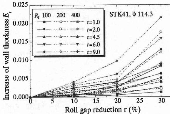
Fig. 9 Effect of  $r$ ,  $t$  and  $R_1$  on  $E_t$ .
