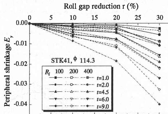
Fig. 5 Effects of  $r$ ,  $t$  and  $R_1$  on  $E_y$ .
