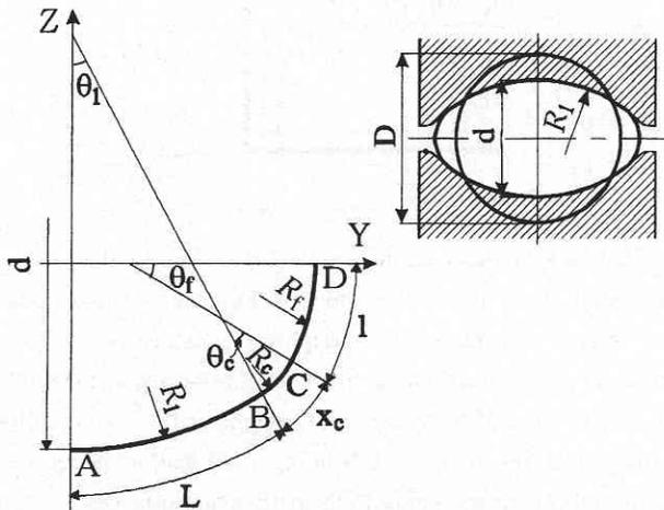
Fig. 2 Geometrical model of cross-section of pipe.
