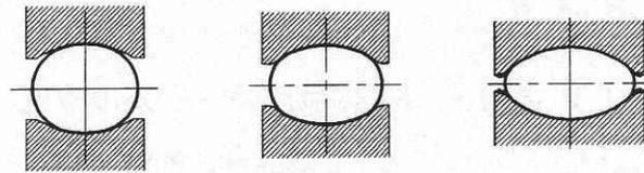
Fig. 8 Cross-sectional diagram of deformed pipe at each step.
