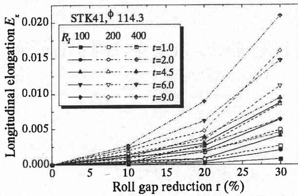
Fig. 6 Effects of  $r$ ,  $t$  and  $R_1$  on  $E_x$ .
