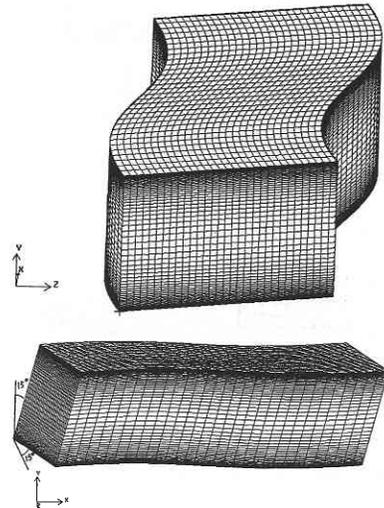
Fig. 3 Curvilinear skew grids for channel flow
