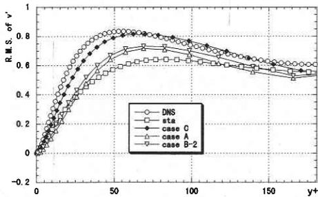
Fig. 7 Intensity of normal-wall wise direction  $Re = 360$
