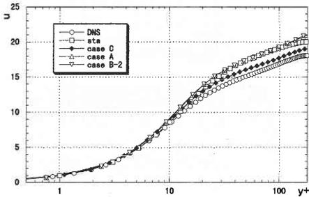
Fig. 5 Main flow velocity profile at  $Re = 360$
