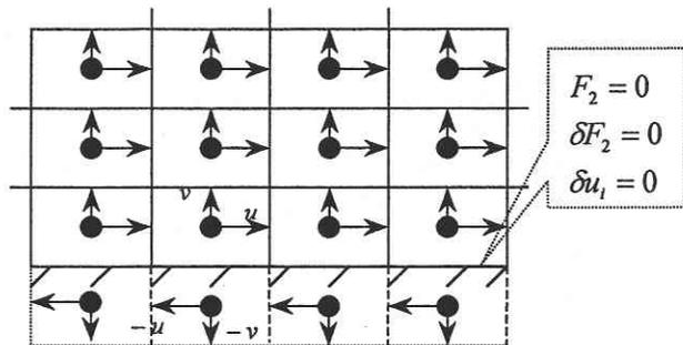
Fig. 4 Wall boundary condition (no slip) in co-located grids system
