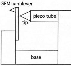
Fig. 1 Schematic of the experiment. An STM tip is positioned against the metal coated surface of a silicon SFM cantilever. Images of the metal coating could readily be observed in the STM mode, but free vibration of the cantilever was prevented by the tip sample interaction.
