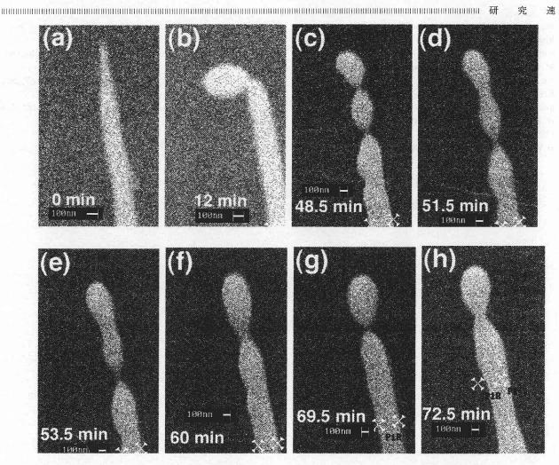
Figure 2 Morphological changes observed when heating a sharpened polycrystalline tungsten tip.
