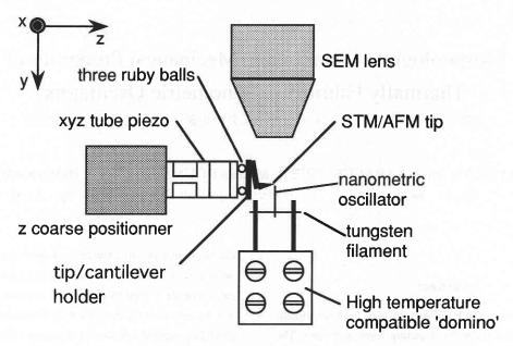
Figure 1 Schematic of the STM/SFM that mounts on a commercial SEM sample stage.
