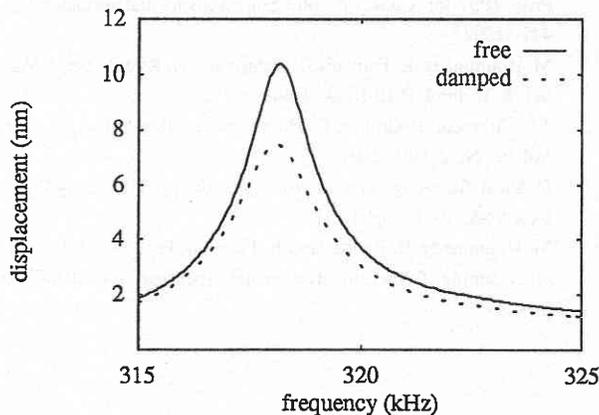
Fig. 3 variation of amplitude due to air damping
