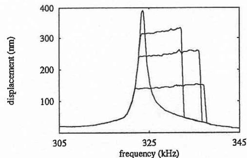
Fig. 6 frequency response obtained with a large amplitude of vibration
