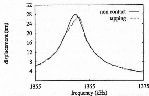
Fig. 5 frequency response for soft tapping mode (second mode)
