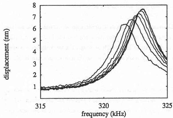
Fig. 4 resonance frequency shift due to Van der Waals attractive forces
