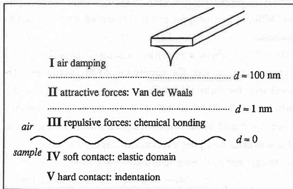
Fig. 2 Different probe-surface dynamic interaction as a function of tip-sample distance  $d$
