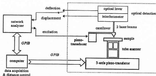
Fig. 1 Force microscope for tip-sample interaction measurement
