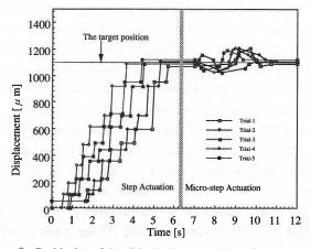
Figure 9 Positioning of the slider in the step and the micro-step actuation
