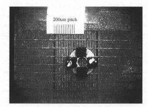
Figure 3 Stator (the electrodes film) and slider which is placed upside down
