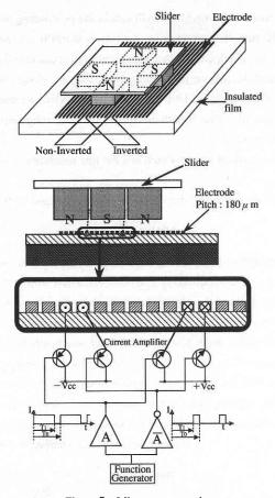
Figure 5 Micro-step actuation
