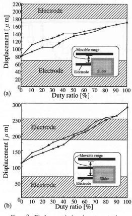
Figure 8 Displacement in the micro-step actuation
