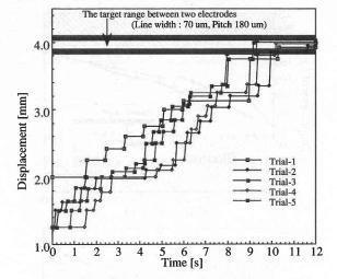
Figure 7 Displacement of the slider in the step actuation
