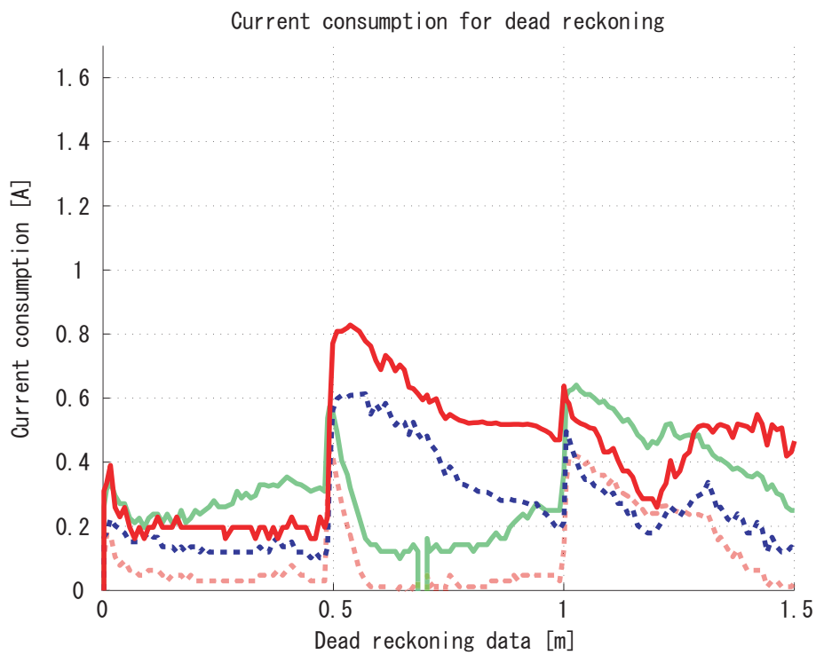
Fig 6.9: Current consumption of wheel motor i (Experiment with movable center of mass)
