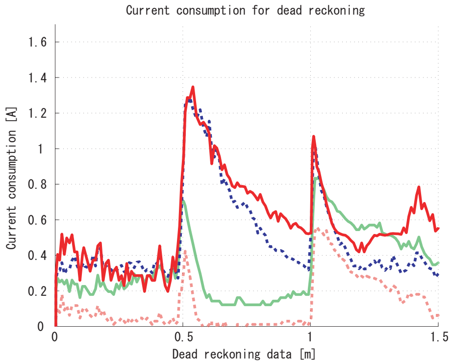
Fig 6.25: Current consumption of wheel motor i (movable mass : fixed mass = 0.33:1)
