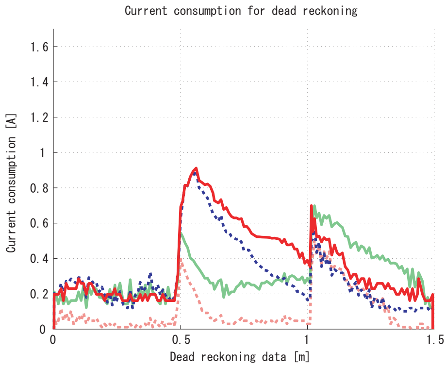
Fig 6.45: Current consumption of wheel motor i (k_a = 0.2, k_s = 0.8)
