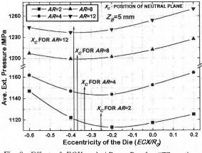
Fig. 8 Effect of ECX and AR on  $P_{Av}$  for "T" sections,  $Z_B = 5 \text{ mm.}$
