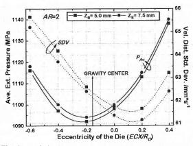
Variation of  $P_{Av}$  and SDV at the die entrance Fig. 4 with ECX and  $Z_B$  for a "L" section, AR = 2.
