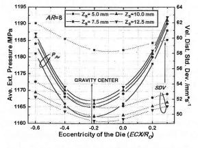
Variation of  $P_{A\nu}$  and SDV at the die entrance Fig. 3 with EC and  $Z_B$  for a "L" section, AR = 8.
