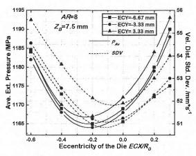
Fig. 5 Variation of  $P_{Av}$  and SDV at the die entrance with ECX and ECY for a "L" section, AR = 8,  $Z_B = 7.5 \text{ mm}.$
