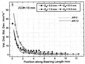
Variation of SDV along bearing length for "T" Fig. 7 sections, ECX = -10 mm.
