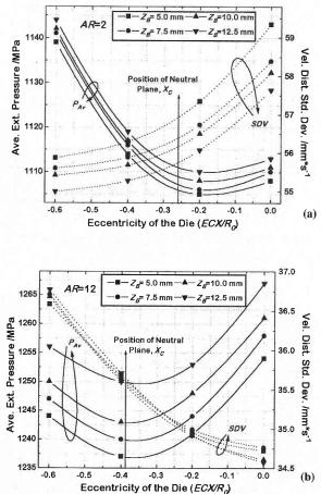
Fig. 9 Variation of  $P_{Av}$  and SDV at the die entrance with EC and  $Z_B$  for "T" sections (a) AR = 12, (b) AR = 2.
