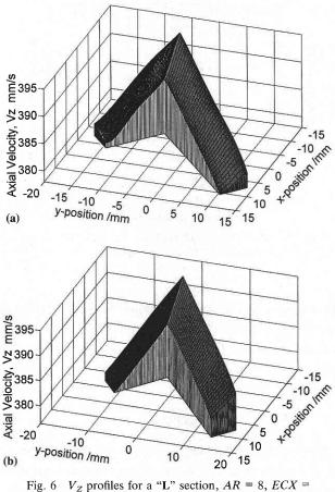
$-10 \text{ mm}, Z_B = 7.5 \text{ mm}$  (a) ECY = 26.67 mm**(b)** ECY = -3.33 mm.
