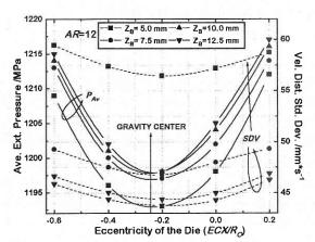
Variation of  $P_{Av}$  and SDV at the die entrance Fig. 2 with EC and  $Z_B$  for a "L" section, AR = 12.
