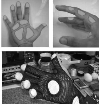
(a) 13 tactile sensors configuration
