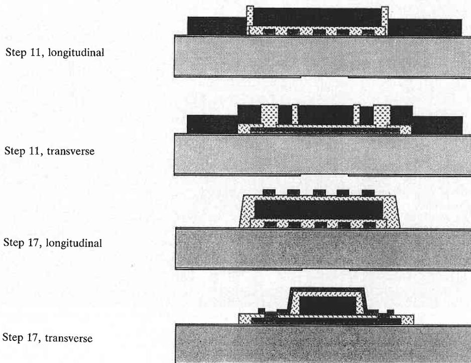
Fig. 3 Longitudinal and transverse cross sections of the coil for process step 11 (electroplating of  $10\ \mu\text{m}$  of permalloy) and 17 (electroplating of the last layer of copper). Horizontal and vertical dimensions not to scale.
