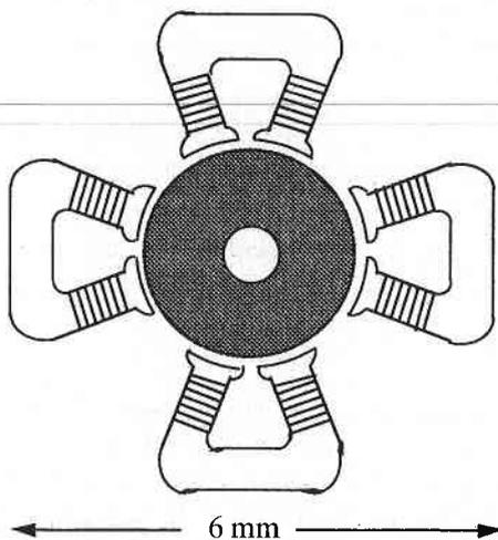
Fig. 1 Layout of rotor and stator. The rotor diameter is 3 mm.
