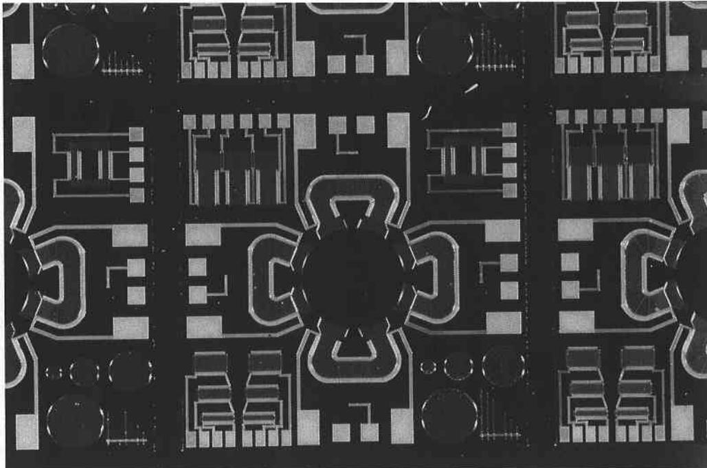
Fig. 4 Photograph of the micromachined batch-fabricated magnetic bearing system. One square unit measures  $1\ \text{cm} \times 1\ \text{cm}$ .
