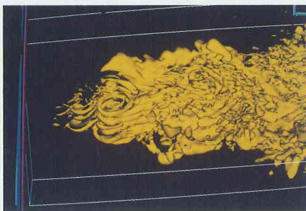
Photo 6. Iso-surface of Vorticity in x-direction \omega_x
