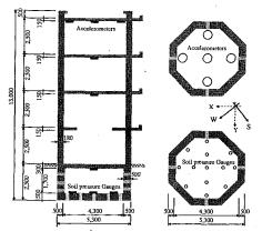
Fig. 1(a) Plan and cross-section of the tower [4]
