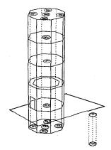
Fig. 1(b) Locations of the Accelerometers
