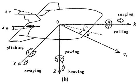
Fig. 1. (a) The "Pteroa-150" Vehicle, (b) Coordinate System
