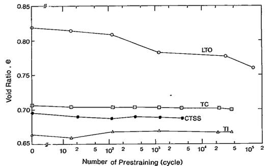
Fig. 11 Number of cyclic prestraining versus void ratio at the end of each cyclic prestraining
