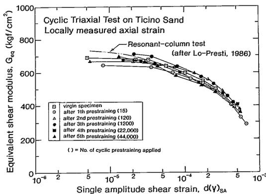
Fig. 7 Effect of cyclic prestraining on stiffness, dense Ticino sand (Test TI)
