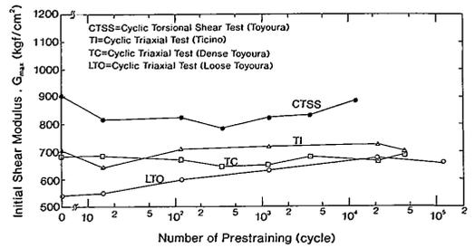
Fig. 10 Initial shear modulus,  $G_{max}$ , versus the number of cyclic prestraining immediately before the measurement of  $G_{max}$ . Note the number of cyclic prestraining shown here is not the accumulated value.
