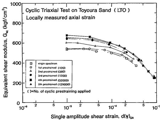
Fig. 9 Effect of cyclic prestraining on stiffness, loose Toyoura sand (Test LTO)
