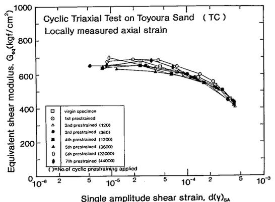
Fig. 8 Effect of cyclic prestraining on stiffness, dense Toyoura sand (Test TC)
