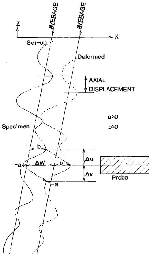
Fig. 4 Error involving the lateral strain measurement
