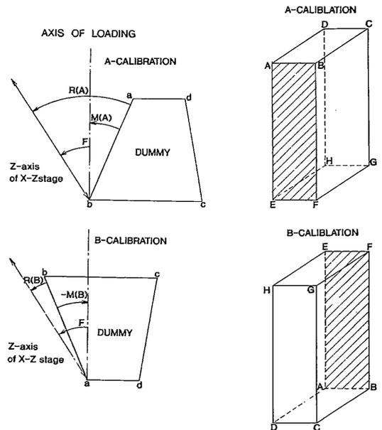
Fig. 5 Calibration to measure the angle between a z-axis of LDMS and the direction of loading.
