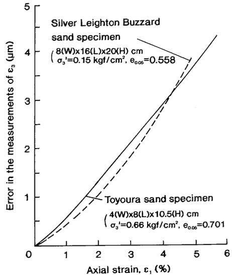
Fig. 6 Error in the measurement of displacement in the x-direction of LDMS in relation to the axial strain.
