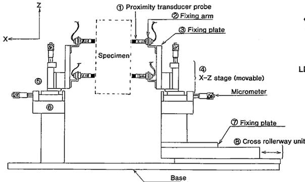
Fig. 2 Lateral deformation measuring system (LDMS).
