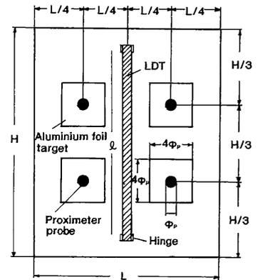
Fig. 3 Positionings of instrumentation for local strain measurements.
