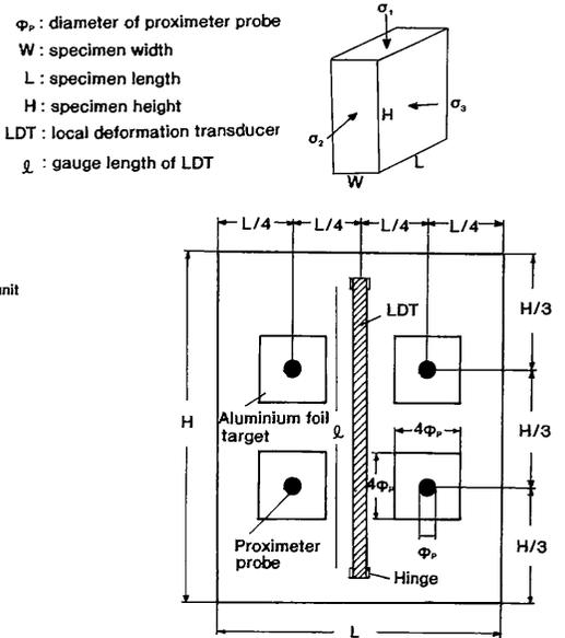
Fig. 3 Positionings of instrumentation for local strain measurements.
