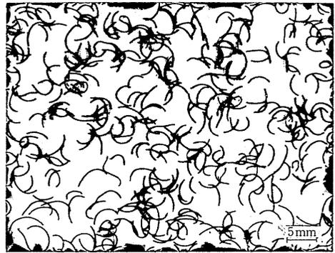
Fig. 8 Samples of φ200μm SiC short fiber
