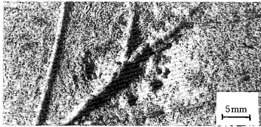
Fig. 5 Defect on the transprinted surface of ZA-27
