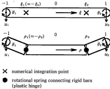
Fig. 2 Cubic beam element and its physical equivalent
