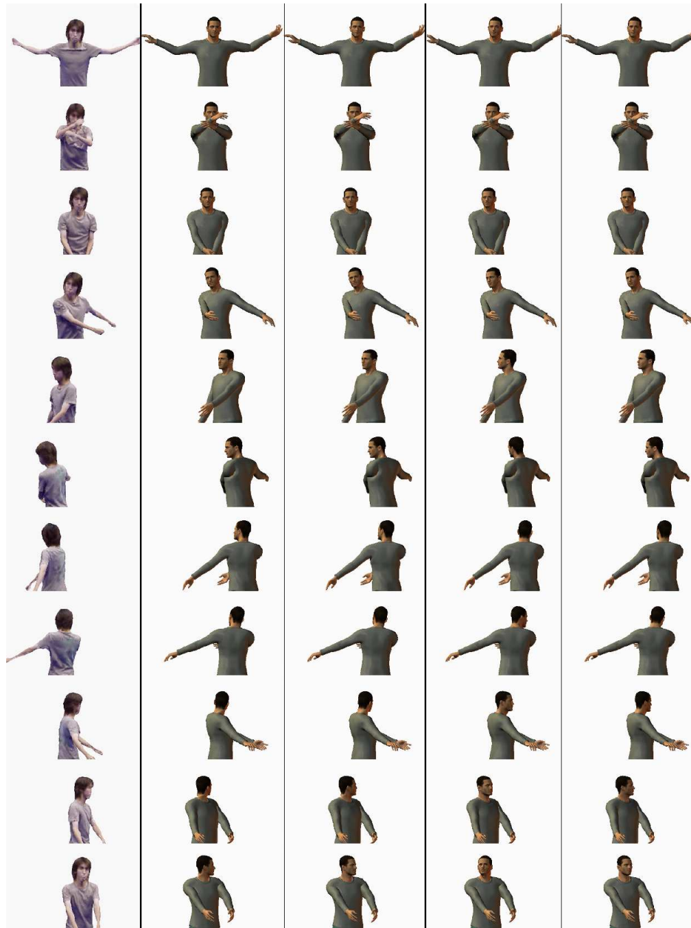
Figure 7.8: (From left column) Original model with color information, 20% vertices with time step = 1, 20% filtered vertices with time step = 5, 10% vertices with time step = 1 and 10% filtered vertices with time step = 2.
