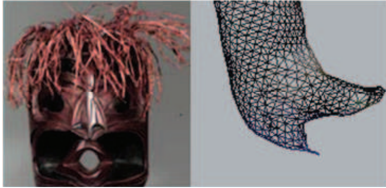
Figure 2.5: Limitations of volume intersection method. (Left) Example of topology that fails [3]. (Right) Example of bad background subtraction.
