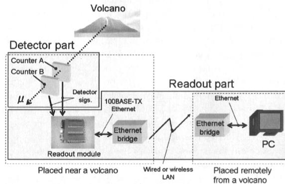
Fig. 1. Detection system for cosmic-ray muon radiography
