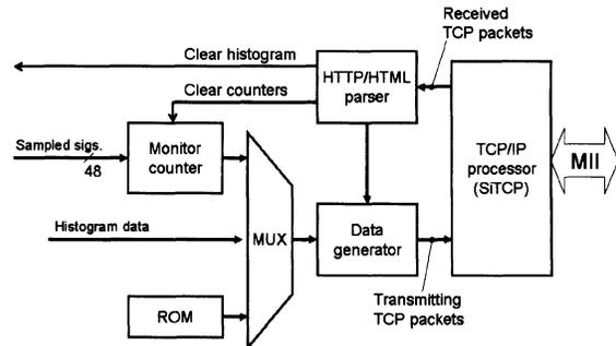
Fig. 6. Block diagram of the network processor.
