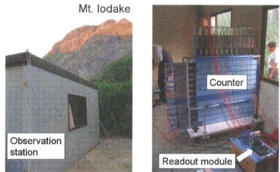
Fig. 9. Photograph of the observation station and detection system. (a) Observation station with Mt. Iodake in the background. (b) Detection system installed in the station (other counter not shown).
