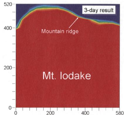
Fig. 10. A radiographic image of Mt. Iodake. The red and blue areas represent relatively high and low density, respectively.
