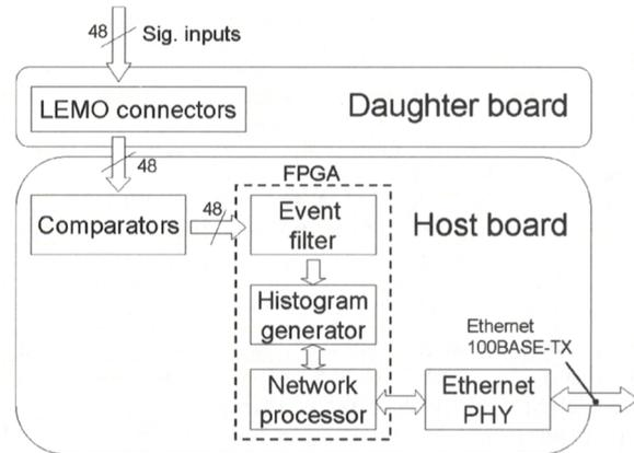
Fig. 4. Block diagram of the readout module.
