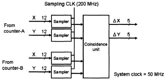
Fig. 5. Block diagram of the event filter
