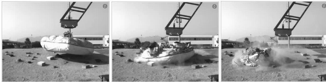
Fig. 2.9: Landing test of Vented Airbag ((c)ESA)
