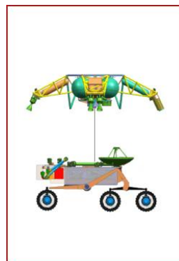
Fig. 2.12: Sky Crane for Mars Science Laboratory ((c)NASA/JPL)
