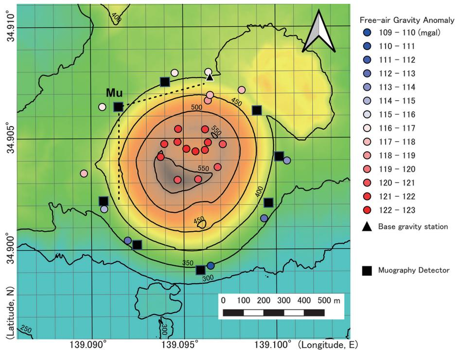
Fig. 2. Locations of gravity stations (circles) on and around the Omuro scoria cone with their colors indicating values of free-air gravity anomaly. Black squares indicate positions of muography detectors. Background color contour map and lines represent the topography of the cone (unit: meter).
