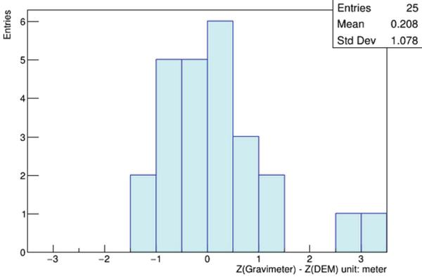
Fig. 3. Comparison between altitude of gravity station determined from the GNSS survey and altitude taken from the digital elevation model (DEM5 A by Geospatial Information Authority of Japan).
