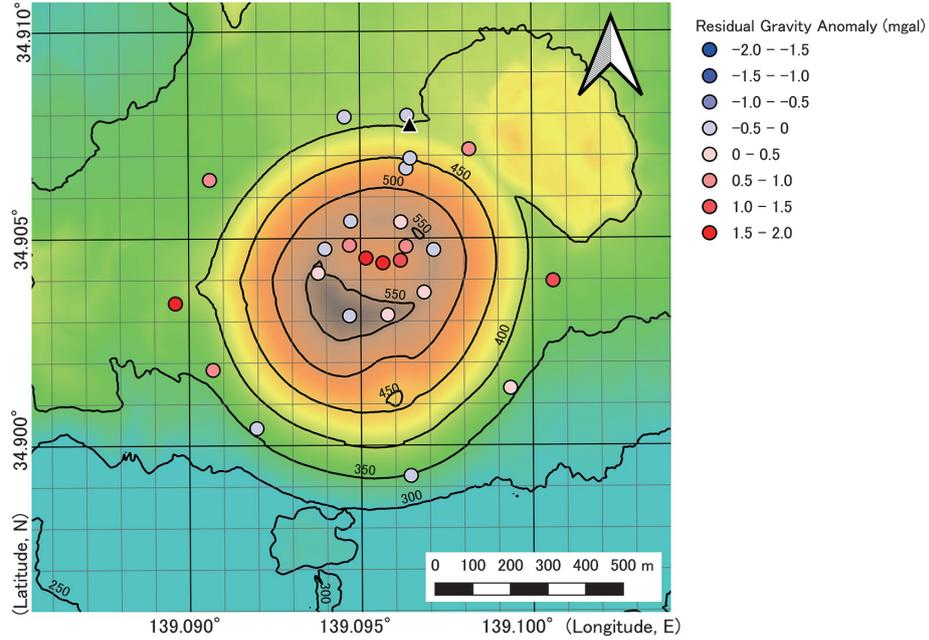
Fig. 4. Residual gravity map after removing the topographic effect (terrain density:  $1.39 \text{ g cm}^{-3}$ ) and the regional trend. The background color contour map and lines represent the topography of the cone (unit: meter).
