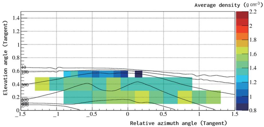
Fig. 5. Two-dimensional density map from muography observations at the northwest foot of the Omuro scoria cone (“Mu” in Figure 2). Color in each rectangular bin represents average density along lines of sight of the detector. Black solid contour lines represent the thickness of the mountain along lines of sight of the detector (unit: meter).
