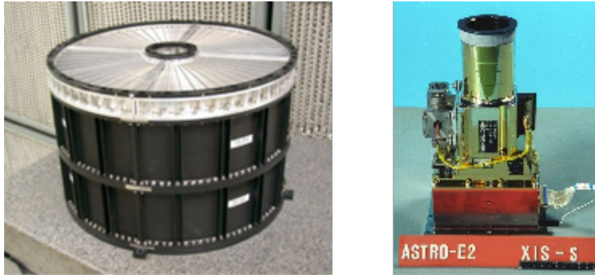
Figure 4.2 Pictures of XRT and XIS onboard Suzaku
