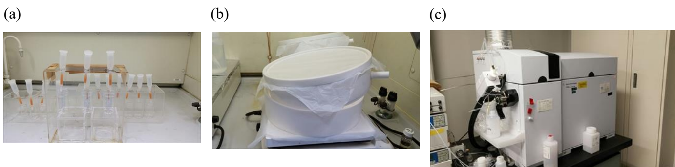
Fig. 5-2. (a) Column processing for extracting REEs. (b) Evaporation to dryness of HNO 3 or HCl covering a PTFE sheet. (c) ICPMS (Agilent 7700cs).
