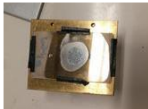
Fig. 3-8. Thin plate amounted the sample with resin, which was coated by carbon. Thin plate was set by carbon tape for SEM observation.
