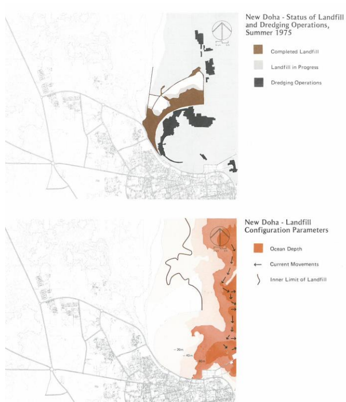
Figure 3.4- New Doha- Status of Landfill and Landfill configuration in 1975 (Pereira Associates, 1975, p.59)
