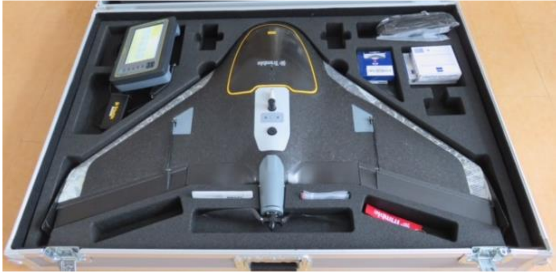
Figure 2.6: Trimble UX5 fixed-wing UAV used in this study and its accessories.
