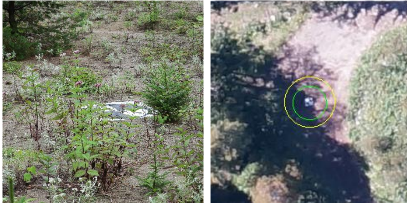
Figure 2.8: View of a GCP on ground (left) and in UAV aerial imagery (right).
