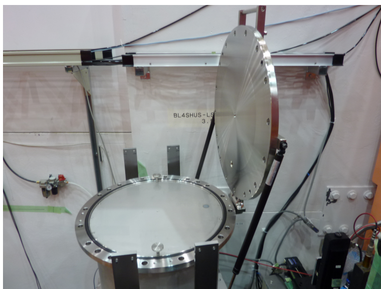
Figure.6.8 Photograph of the storage container with top cover opened. The upper lid of the storage container was opened and the picture was taken from above. The white disc on the top of the cylindrical container is the test material.
