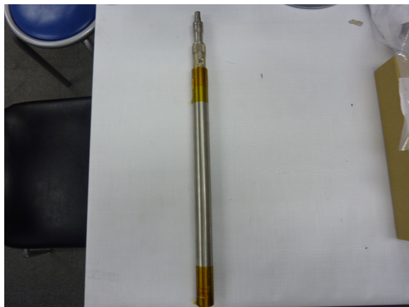
Figure.6.15 RS-P4-0812-223. (Left) Overall image of RS-P4-0812-223 (right) Drawing of RS-P4-0812-223. The chamber of RS-P4-0812-223 is made of SUS304. There is no leakage gas because the joint part is welded.
