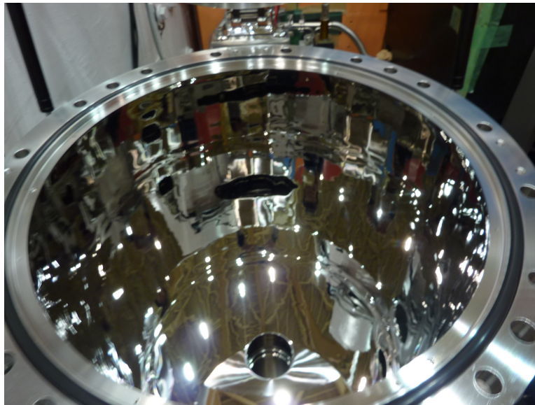
Figure.6.9 Photograph of the inside of the storage container. The upper lid of the storage container was opened, the test material was removed, and the picture was taken from above. The inner surface is subjected to the composite electrolytic polishing treatment and the inner surface is lustered like a mirror.
