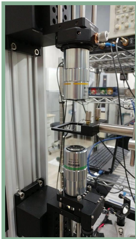
Figure 5.12. A picture of the new microspectrophotometer confocal arrangement, exemplifying a more spacious sample environment.
