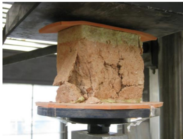
Figure 4. 18. A sample of Brick from Demolished Buildings under Compression Load
