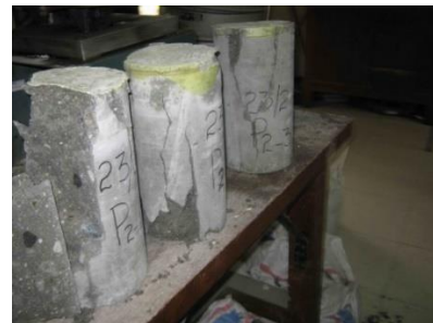
d. Concrete Cylinder after Compression Strength Test
