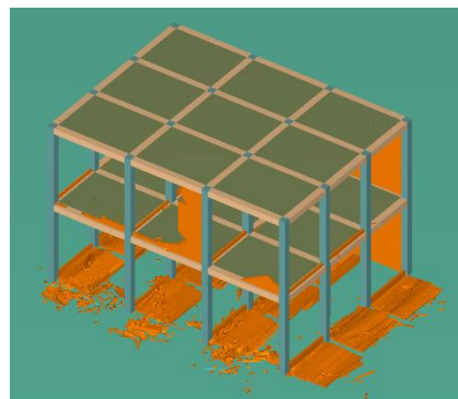
Figure 5. 32. Damage Patterns and Damage Level at 0.4g of Kobe ground motion for RC building Type A with strong (28) concrete strength
