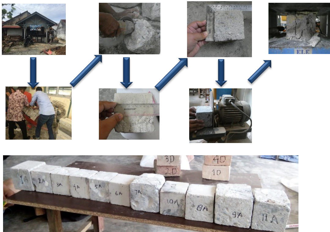
Figure 4. 9. The process of Concrete Cube Sampling from Demolished Buildings
