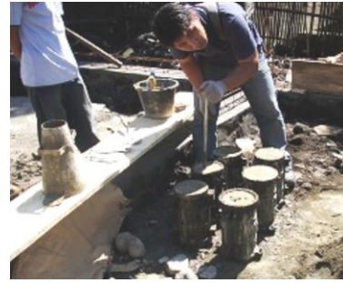
b. Process of Compaction for Casted New Concrete
