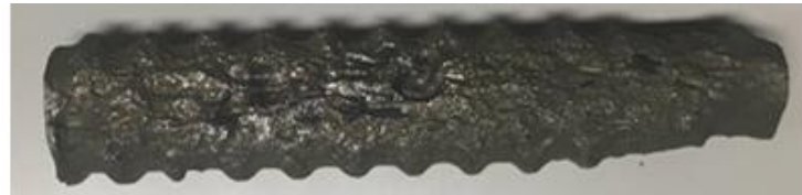
(b) 2 weeks corrosion deformed rebar
