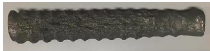
(c) 4 weeks corrosion deformed bar
