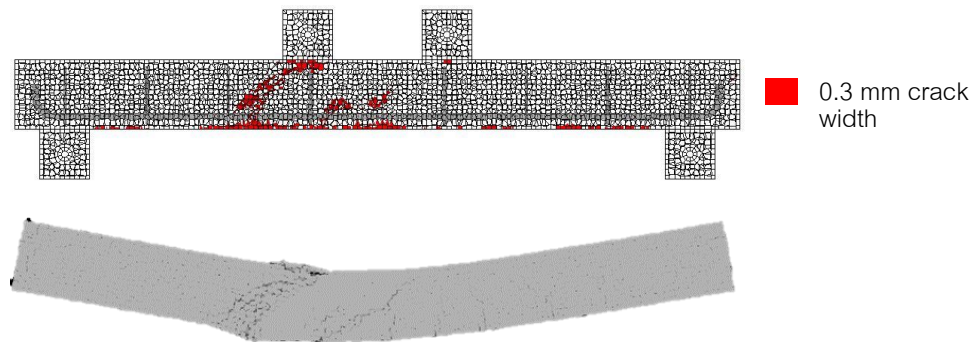
(c) Non-uniform corrosion beam
