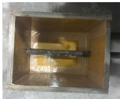
(b) Formwork of corroded reinforcement specimen
