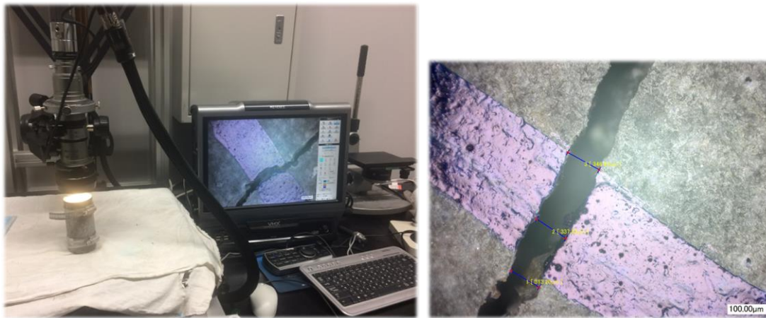
Figure 3.5 Measurement of bottom surface crack width by microscope (a) Crack width measurements along three random points around the markings (b)
