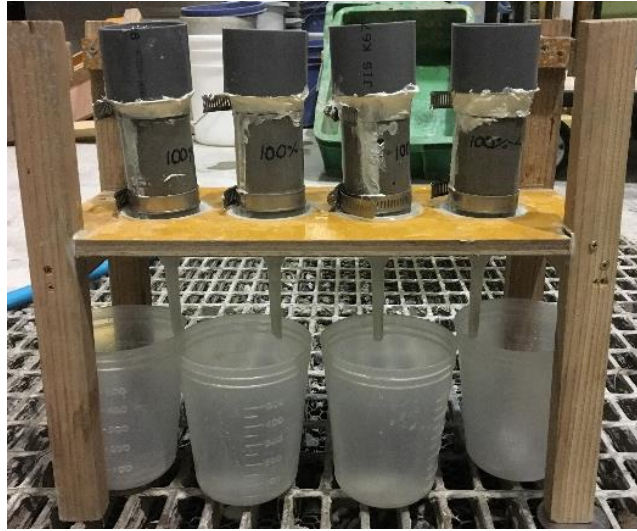
Figure 3.11 Water flow measurement setup
