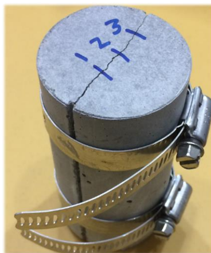
Figure 3.4 Tying back specimen halves and marking of the bottom surface
