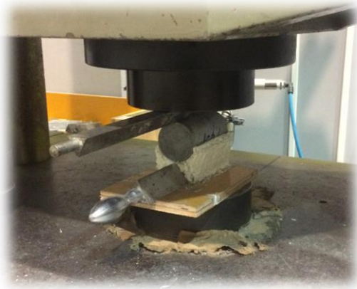
Figure 3.2 Cracking specimen into halves using V-notches
