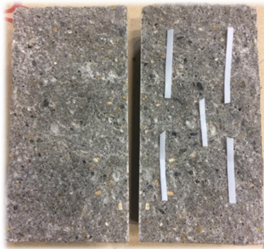
Figure 3.3 Provision of Teflon sheets on crack surface
