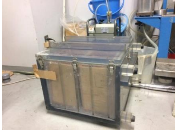
Figure 3.10 Vacuuming of specimen in vacuum chamber
