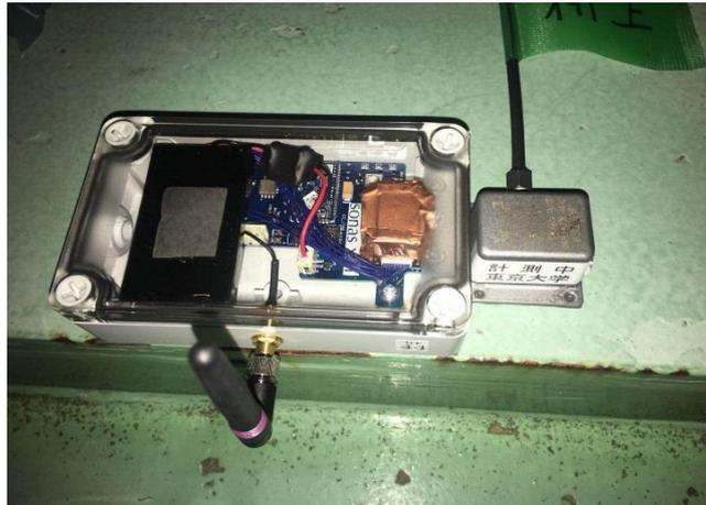
Fig. 6-13. Accelerometers on Yokohama Bridge
