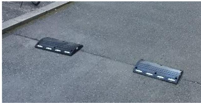
Fig. 3-17. Portable humps for vehicle parameter calibration
