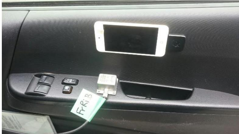
Fig. 3-22. Sensors on the test vehicle
