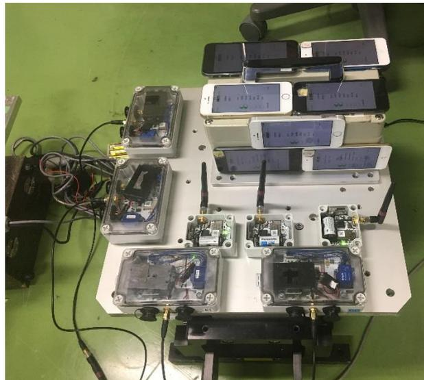
Fig. A-6. Sensor layout of the shake-table test
