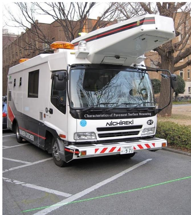
Fig. 1-4. Inertial laser profiler (Nichireki Corporation)
