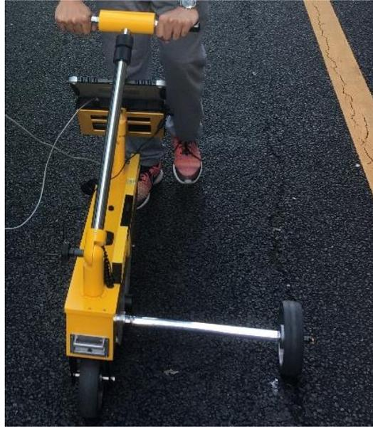
Fig. 4-9. Portable pavement profiler (Suntop techno Corporation)
