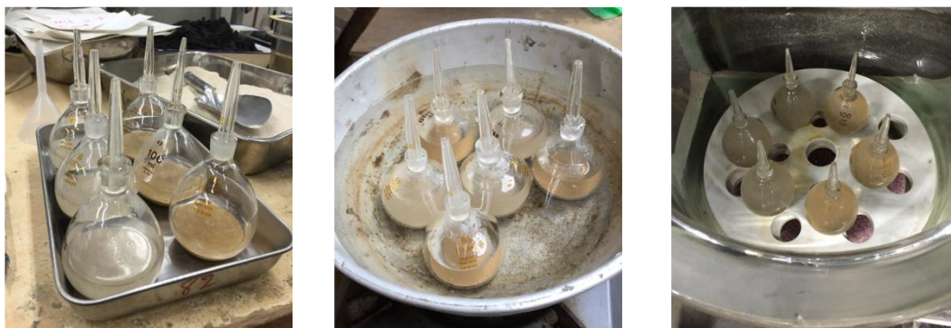
Fig. 3-2 Density bottle method to Determine the Gs
