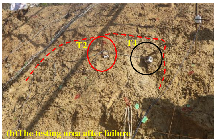
Fig. 6-97 Images of the testing area before and after the slope failure
