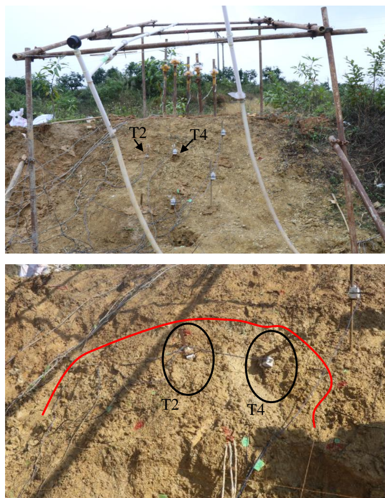
Fig. 7-12 The image before and after the slope failure in Test 4
