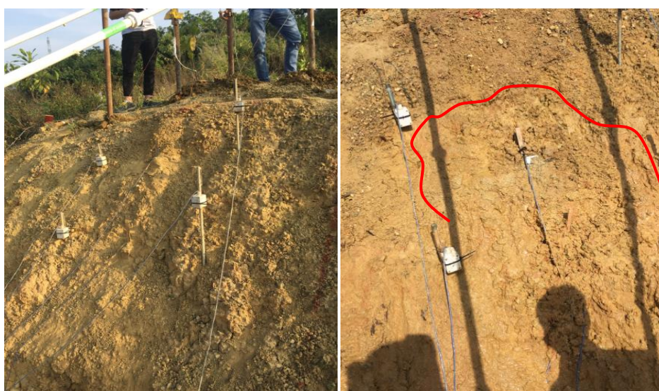
Fig. 7-9 The image before and after the slope failure in Test 3
