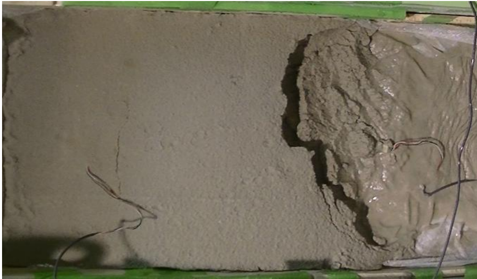
Fig. 7-24 The image of T2 damaged by erosion
