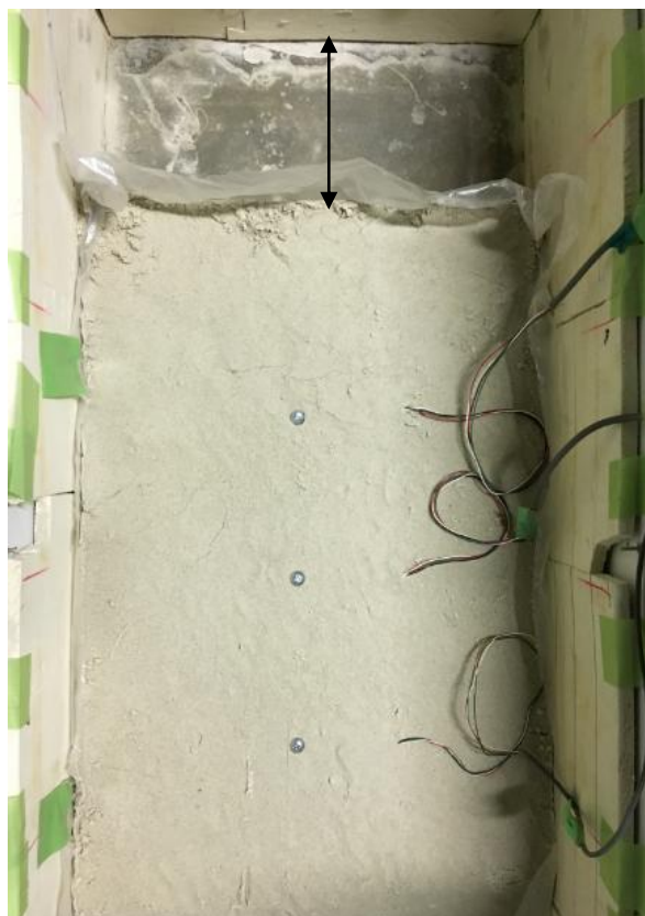
Fig. 5-24 The image of slope failure in Test 10
