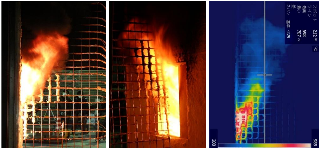
Chamber1-n=1.12-600 kW (a)
