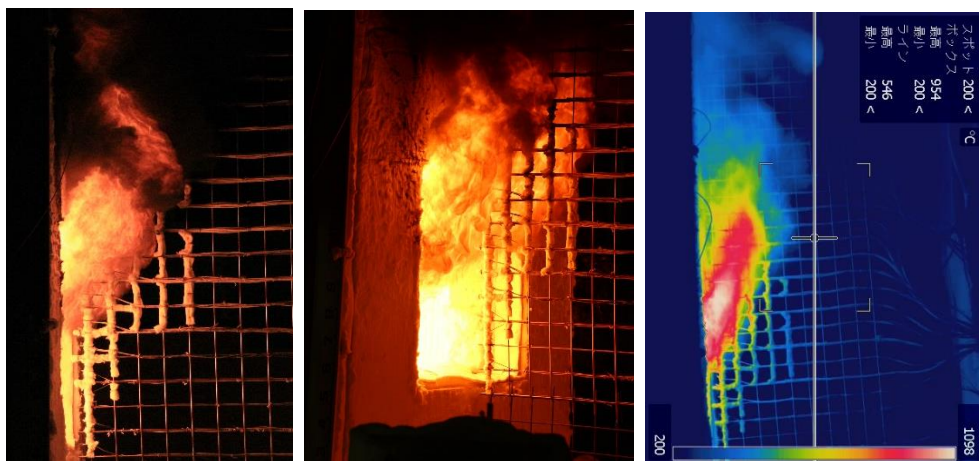
Chamber1-n=2.00-900 kW (a)
