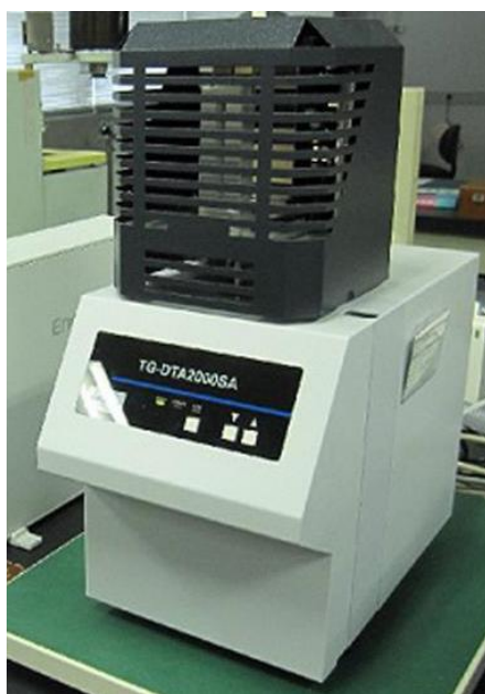
Fig. 8 The description of TG facility
