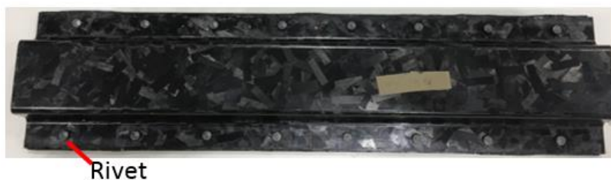
Figure 3-2 Rivet joints for assembling hat-shaped hollow beam
