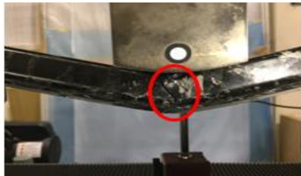
Figure 3-8 Fracture process: crack propagation
