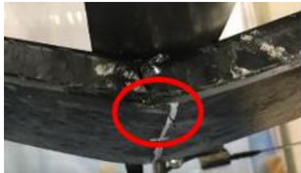
Figure 3-9 Fracture process: tensile failure
