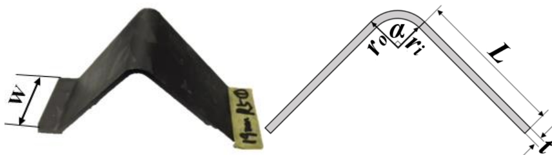
Figure 2-25 Image (left) and dimensions (right) of a representative L-shaped specimen.
