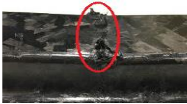
Figure 3-7 Fracture process: compressive fracture
