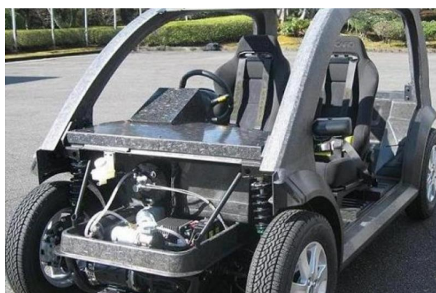
Figure 1-11 47 kg weight cell structure made by random chopped CFRTP [17]
