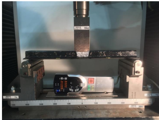
Figure 3-4 Three-point bending test for hat-shaped hollow beam
