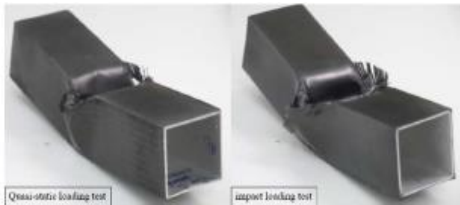
Figure 1-31 Comparison of collapsed specimen under quasi-static (left) and impact loading (right) [53]
