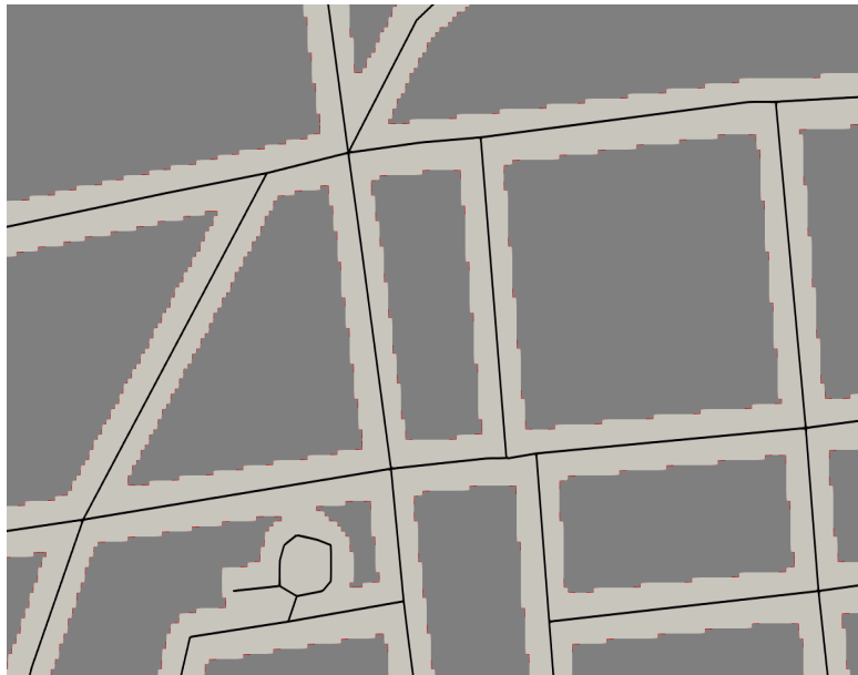
Figure 5.10: The enhanced topological graph from new domain generator.
