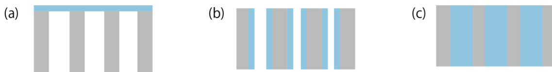
Figure 2.23. Schematic cross-section depiction of (a) membrane surface-functionalized, (b) pore surface-functionalized, and (c) hydrogel pore-filled membranes.
