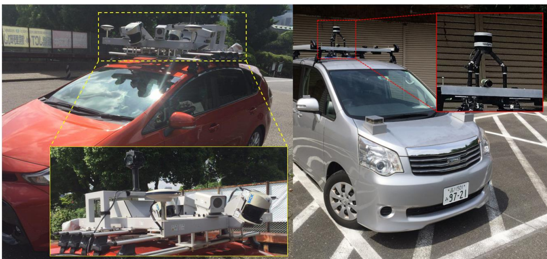
Figure 4-13. The experimental setup. The left is the MMS used for the mapping and the right is our experimental vehicle. Velodyne VLP-16 is mounted on the top of this car at a height of 2.3m.
