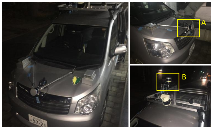
Figure 6-2 Our experimental vehicle. Front Velodyne VLP-16 is used for mapping and it is tilted to scan the environment densely (pitch -80^\circ ). Top VLP-16 used for localization.
