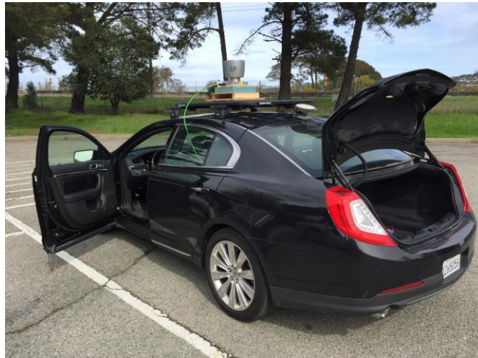
Figure A. 3. The designed data collection platform for autonomous driving
