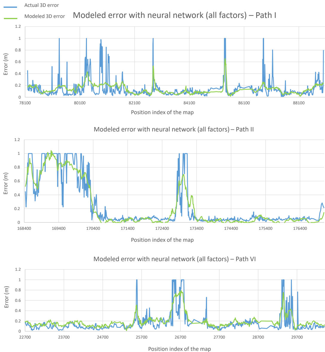
Figure 6-12 Modeled error (green) vs actual error (blue) for the path #I, #II, #VI.
