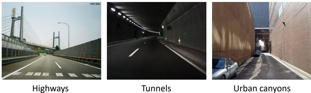
Figure 5-6 Situation that the map does not have any lateral feature to get the longitudinal position.
