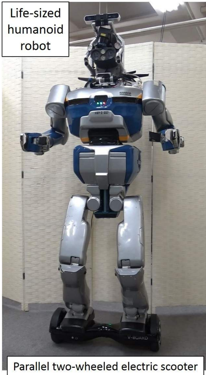
図 6.14: Speed Governing Behavior of Life-Sized Humanoid Robot on Parallel Two-Wheeled Electric Scooter
