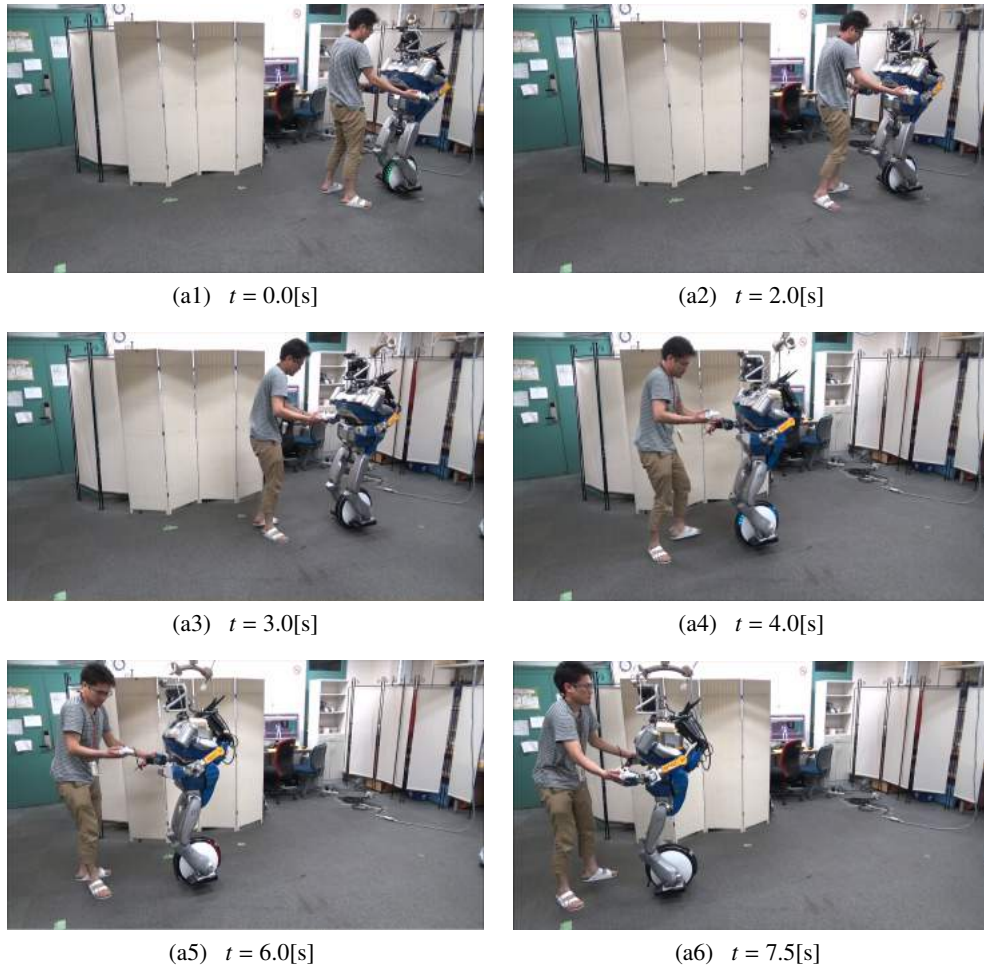
図 7.12: Experimental Snapshot of Driving “Ninebot One S2” without Training Wheels by Life-Sized Humanoid Robot
