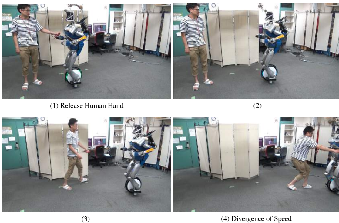
図 7.7: Behavior of Life-Sized Humanoid Robot on “Ninebot One S2”
