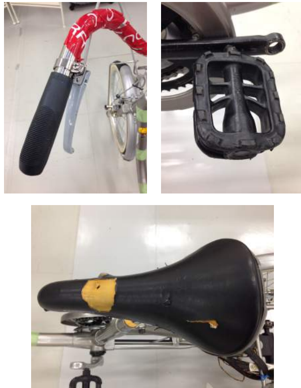
図 A.3: Left: Handle Grip Rubber of Tricycle, Right: Plastic Pedal of Tricycle, and Bottom: Urethane Saddle of Tricycle
